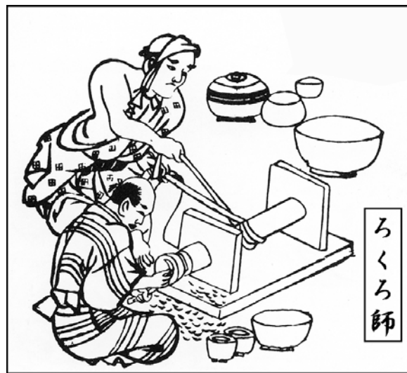
Fig.5 Scene of wood turners at work using a turner: Wakoku-shoshoku-ezukushi (occupations in Japan expressed in pictures) (1685) (3)
