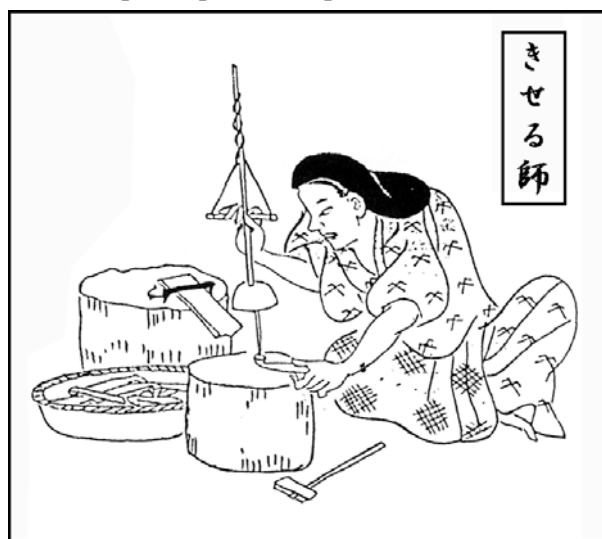
Fig.6 Scene of drilling a hole by a tobacco pipe maker using the Archimedean drill: Imayo Shokunin-zukushi Uta-awase (1821) (3)
